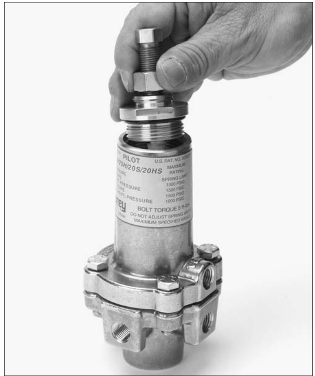
Figure 18 - Installing the closing cap assembly for Pilot with the Red, Cadmium, Blue, and Purple Springs.
