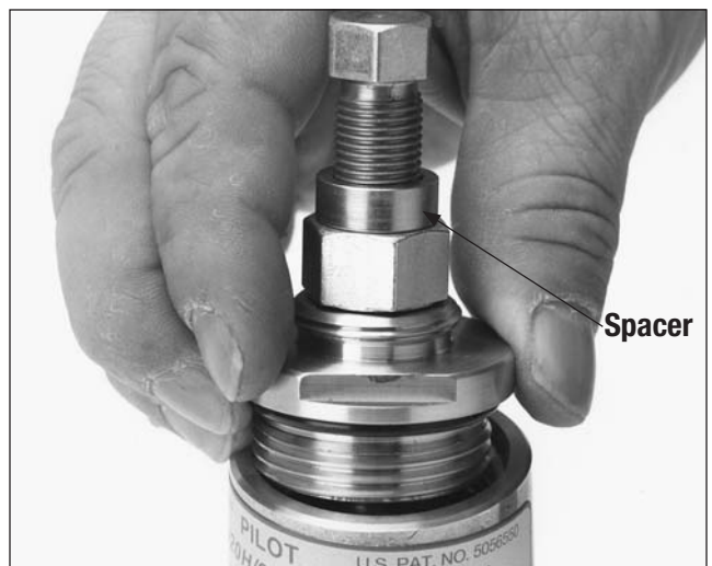
Figure 19 - Installing the closing cap assembly with spacer (to prevent spring over compression) for Pilots with the Black and Green Springs.
