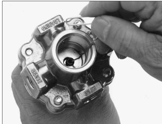
Figure 12 - A paper clip easily pops the O-Ring out of the pilot body.
