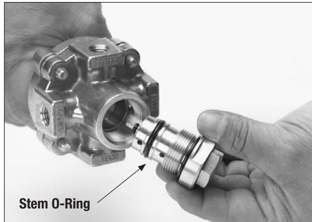
Figure 25 - Insert Body Insert (Cartridge) with lubricated Stem O-Ring into the Pilot Body.
