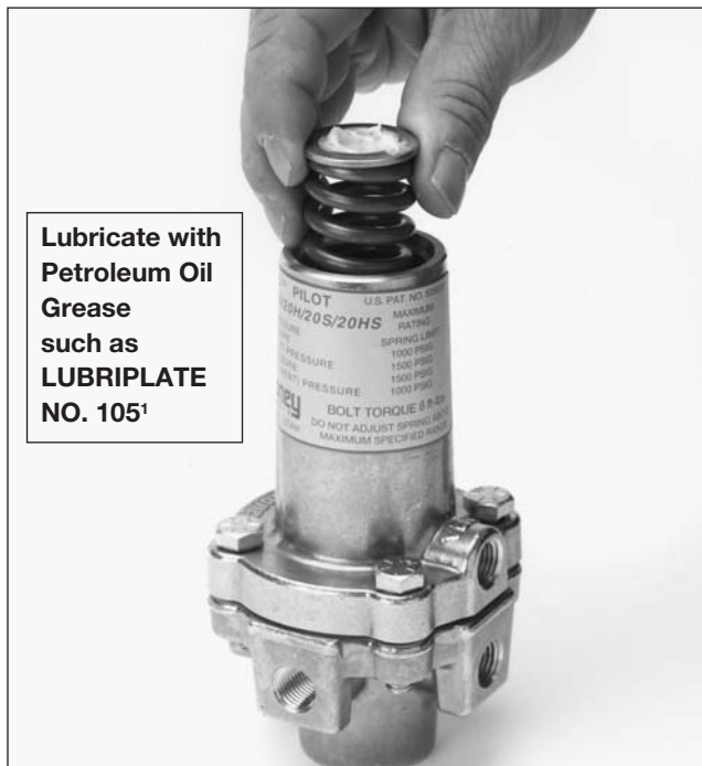
Figure 17 - Installing the Spring with lubricated Spring Follower.
